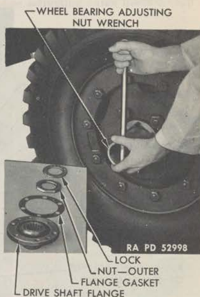
Figure 153—Adjusting Front Wheel Bearing
