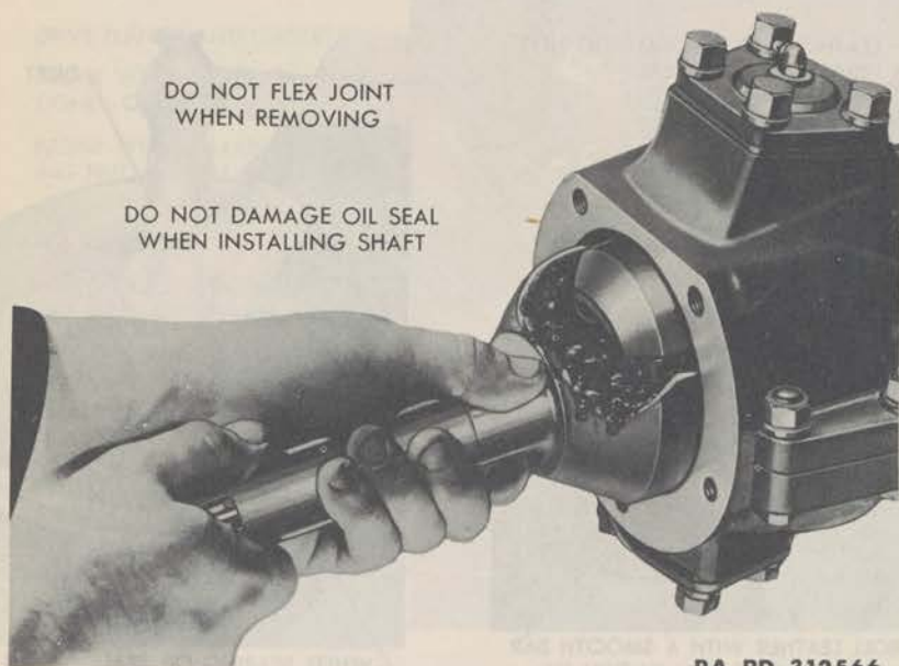
Figure 157—Removing Universal Drive Assembly
