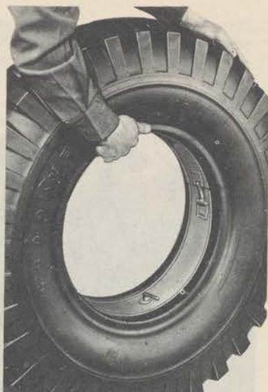
TIRE BEAD LOCK RING INSTALLED
