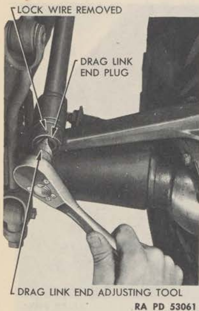
Figure 190—Adjusting Drag Link End
