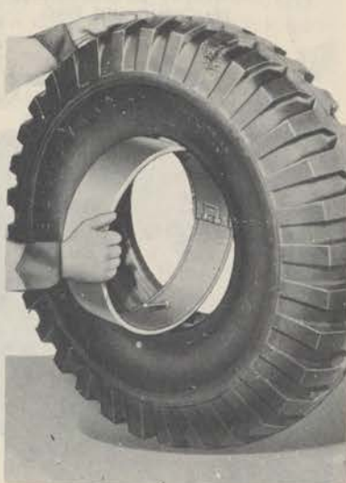
SLIDING TIRE BEAD LOCK RING ON VALVE STEM
