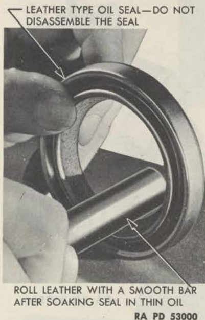
Figure 155—Conditioning Oil Seal
