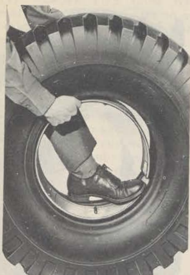
EXPANDING TIRE BEAD LOCK RING IN TIRE
