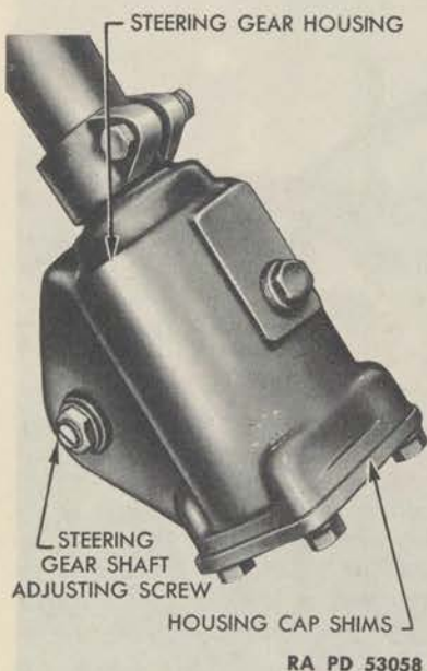
Figure 186—Worm and Shaft End Play Adjustments
