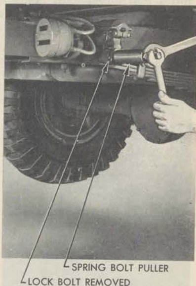
Figure 199—Removing Rear Spring Shackle Bolt with Puller 41-P-2951-70
