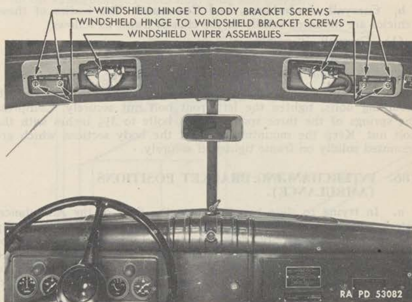
Figure 203—Windshield Hinge and Wiper Location (Closed Bodies)
