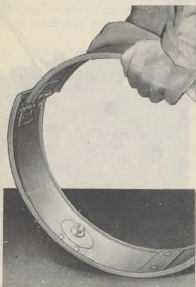
COLLAPSING TIRE BEAD LOCK RING
