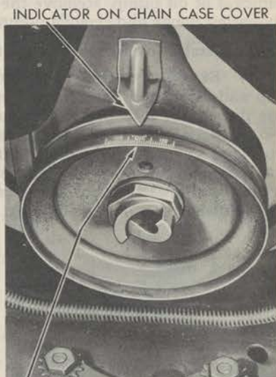
2—LOCATING TIMING MARK ON FAN PULLEY
