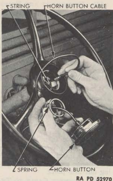
Figure 133—Installing Horn Button Cable
