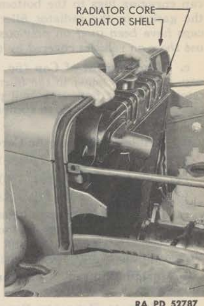
Figure 97—Installing Radiator Core
