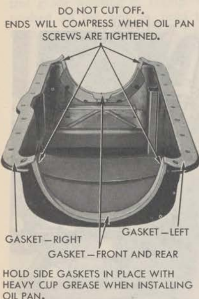
Figure 67—Oil Pan Gaskets
