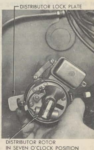
Figure 111—Installing Distributor
