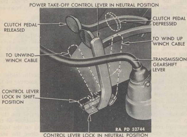
Figure 27—Winch Control Lever Positions
