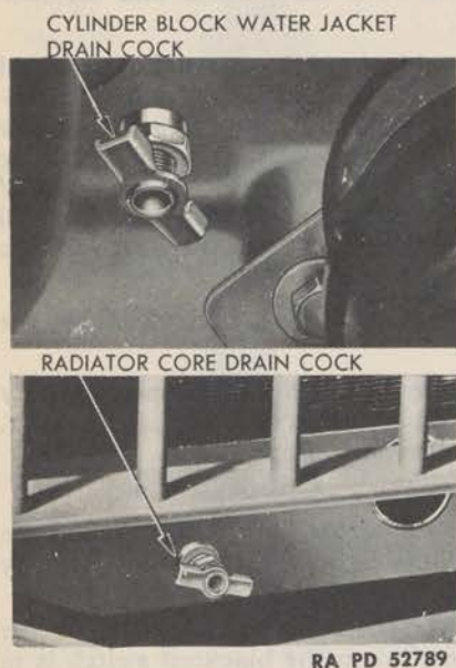
Figure 17—Cooling System Drain Cocks
