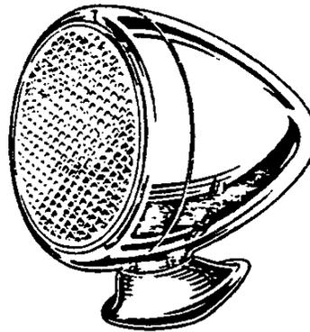
The appearance of the cowl lamps on the sport models is improved to match the headlamps. They too have an embossed bead at the inside edge of the rim which terminates in a sharp point.
